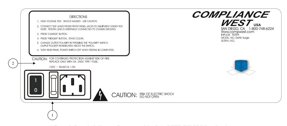
Figure 2. Controls, Indicators, Connectors – MegaPulse DEFIB SURGE P Rear Panel
