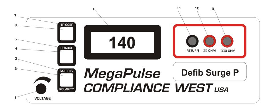
Figure 1. Controls, Indicators, Connectors - MegaPulse DEFIB SURGE P Front Panel
